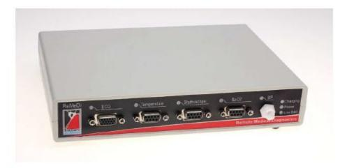
As the name suggests this unit is connected to all diagnostic devices. This acquire the data and processes the same for onward transmission to the Communicator box. This unit is connected to power source.
